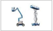
EMERGENCY PROCEDURE: person on the ground activates the emergency rescue button on the base of the machine to bring the basket safely to the ground; SAS rescue from height procedure; SAS notifiable event procedures, SAS general emergency procedures
